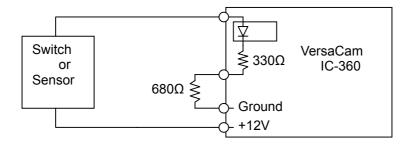
Alternately, a device may supply its own voltage to activate the opto-couplers. For additional details on such circuits, please refer to the pin-out and interface information at the end of this document.
